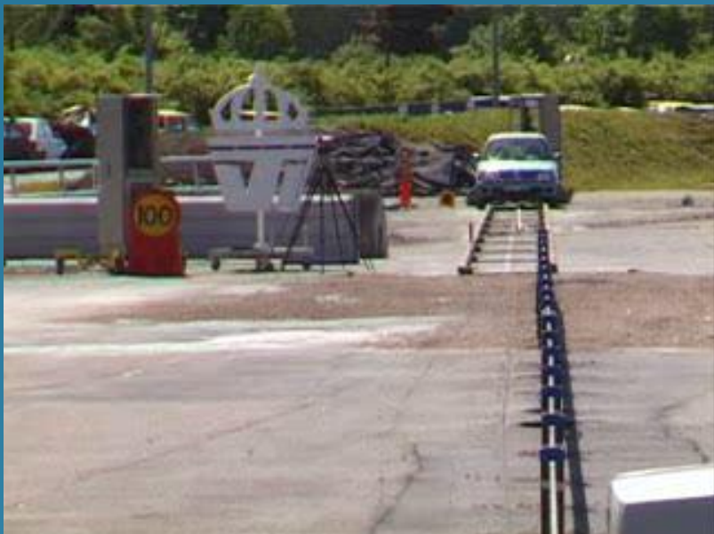
Wire Rope Barrier Ends are Slope Down
